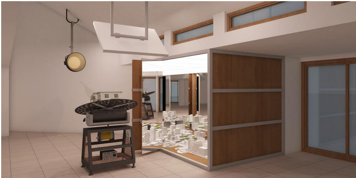
Figure 13: Artificial Clear Sky and Mirror Box
