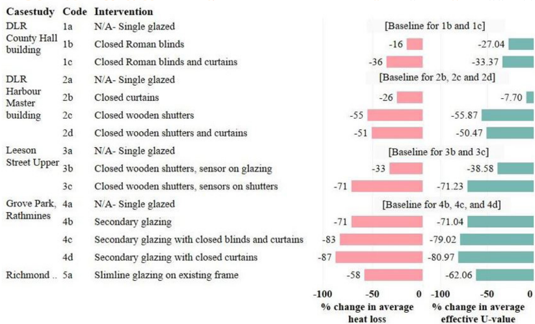
Figure 1: Change in heat loss through the surface and effective U-value for each intervention broken down by case study. All changes are relative to the respective single-glazing baselines.
